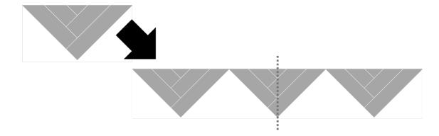
• Start connecting the sets and laying the first row from the left side, using A plank. The long side should be connected at an angle, and the short side should be tapped with a rubber mallet. Repeat the same process towards the right until the row is completed. Cut the planks appropriately at the ends of the room. Don't forget to leave a 6 mm gap near the walls.
