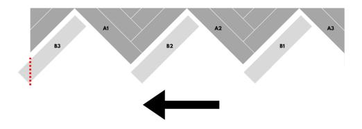
• To finish up the installation, repeat the same process cutting the planks accordingly at the end of the room. Do not forget to leave 6 mm (1/4") of gap from the wall.
