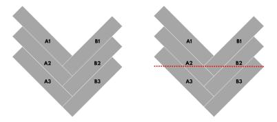
Once you make the first set, you can cut additional sets by following the same process. The number of starting sets depends on the width of your room. Cut the starting sets accordingly at the end of the room. Do not forget to leave 6 mm (1/4") of gap from the wall. Line up starting sets using your main axis and align properly, so they can be connected together.
