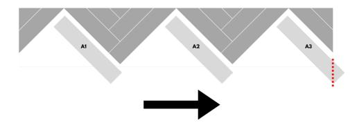
• Start the second row from the right side using B plank. The long side should be joined at an angle, and the short side should be tapped with a rubber mallet. Repeat the same steps towards the left until the row is completed. Cut the planks appropriately at the ends of the room. Don't forget to leave a 6 mm gap near the walls.
